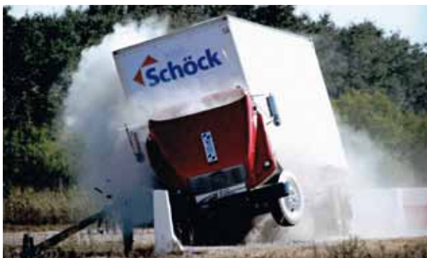
Successful crash test on TL-5/Pl-3 barrier wall College Station, TX, USA
