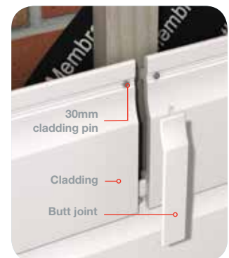
Diagram 8 For continuous runs, a butt joint connects the cladding. This is staggered per length and positioned where a vertical batten is located
