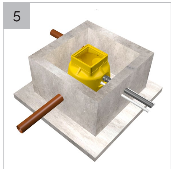
Position chamber in RC box.
