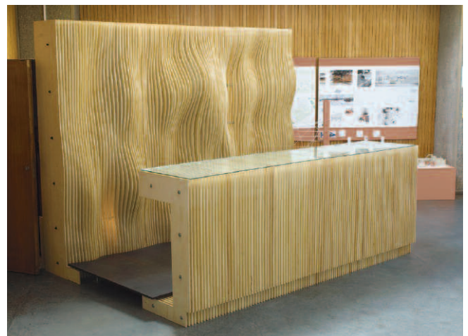
'Centenary Bar' at Sheffield University's School of Architecture, CNC machined Grade S/BB Birch Plywood with WISA-Hexagrip floor.
