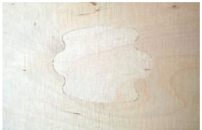
A 'Batman' shaped plug or patch – often found on BB Grade Plywood. These patches are well made and give a sound/solid face.
