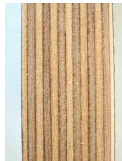
The standard veneer thickness for most European Birch plywood is 1.4mm. Plywood normally has a balanced construction of alternating cross and long grain veneers, i.e. 9-ply for 12mm, 13-ply for 18mm, as can be seen here.
