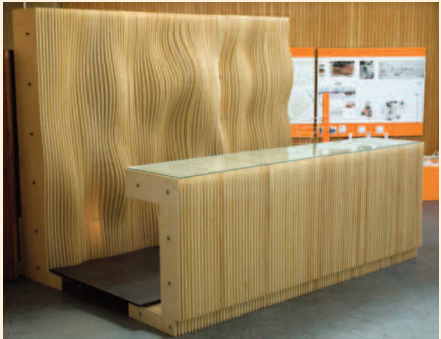
CNC Contoured Birch Plywood Designed by Lukas Barry (University of Sheffield)
