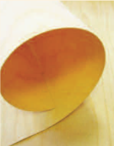
CNC Contoured Birch Plywood Designed by Lukas Barry (University of Sheffield)
