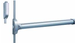
Push bar with choice of single, two- and three-point locking. Vertical locking shoots are concealed in a surface-mounted housing. Easy to specify and install. Incorporates automatic deadlocking.
