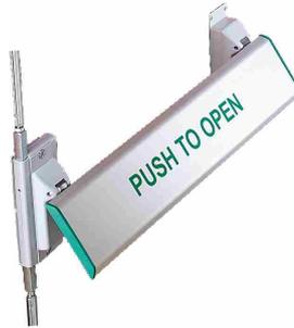
Panic bolts with choice of push pad or plate operating vertical or three-way locking shoots. Supplied with top socket, strikes and dust-excluding floor socket.
